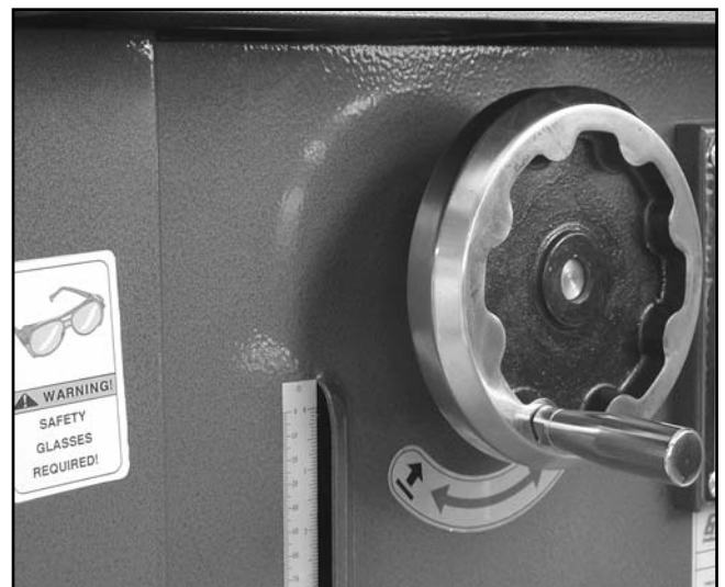
Figure 4. Handwheel mounted to shaper.
